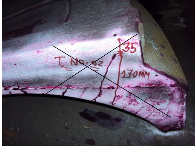
Photo: 3 Example of unacceptable crack at side face on table segment. Total thickness of table segment is 205 mm. Extension of crack is beyond 0.7 times of total thickness of table segment.
